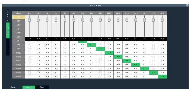
The OUT channel of the mixer is equipped with a gain fader, which allows you to individually control the gain of any output channel with a gain range of (12~-72dB).
