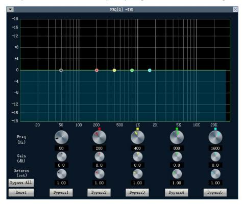
Bypass All/Active: Bypass All or Active the Parametric Equalizer for the current channel; When the Parametric Equalizer is bypassed, audio is passed through without any change;
