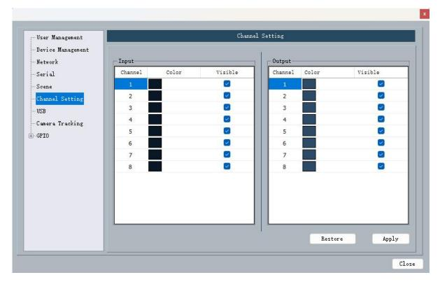
Users can customize the input/output channel UI colour scheme according to the usage scene.
