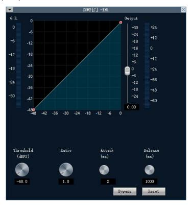
1 Threshold (-48~0): Sets the level where compression begins. This is the point from which the amount of attenuation is calculated based on the Ratio setting. Assuming only one Input, a level below the Threshold Level is not compressed, anything above the Threshold Level attenuation is applied;
