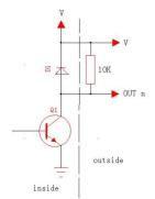
Firstly, connect a 10K/0.25W resistor between a GPIO pin (e.g. port 2) and "V" on the device (as shown in the figure), the pin will output a low level 0 or a high level 1 according to the change of matrix state, and the level can be used to trigger another GPIO or other devices.
