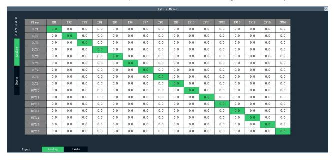
Matrix both signal routing and mixing double multiplexing function, X-axis is the input channel, Y-axis is the output channel, the matrix initialization state is (as shown in the figure above: one-to-one) input and output.
