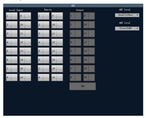
Acoustic Echo Canceler: Set the signal that needs to be processed by the Acoustic Echo Canceler, and the processed signal selects the output channel in the Mixer;
