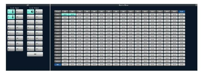
The signals from input channels IN1 and IN2 are processed in the AFC and output in output channel OUT1, configured as shown above:
