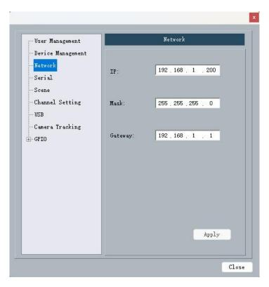
To view and modify the network address information of the device, enter the Network window, type in the IP address, subnet mask and gateway in the corresponding input boxes, and click the [Apply] button to complete the modification.
