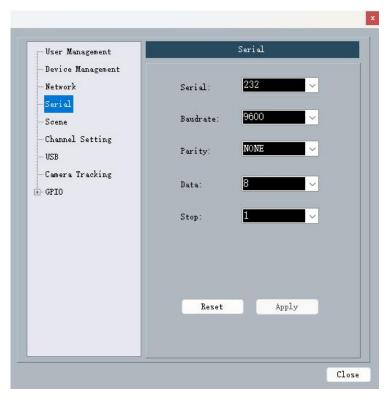
Serial window can view or modify the RS232/RS485 serial port number baud rate, check bit, data bit, stop bit settings are complete, click on the [Apply] button to modify the current device's serial port information, such as the need to restore to the initial default value, click on the [Reset] button, you can restore the settings of the parameter can not be empty.
