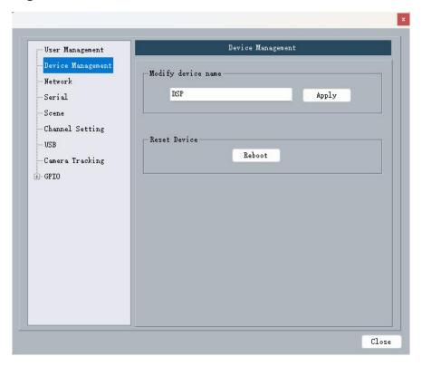
View and modify the name of the device, enter the name of the device in the corresponding location, click the [Apply] button to complete the modification, [Reboot] can be in the window to control the device restart.
