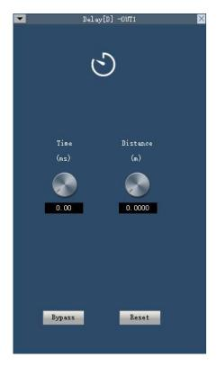
The time interval between the input of a signal to this processor and the output of this processor is generally used to produce other effects such as reverberation or echo, and can equally be used to act as a treatment for auxiliary loudspeakers in larger rendition situations.
