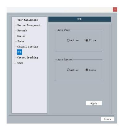
Users can customize to enable or disable the automatic playback/recording function according to the use of the scene, configure the playback channel or recording channel matrix routing in the matrix mixing interface and save the current scene, the device will automatically playback and record after powering on the device again, no need to manually configure separately.
